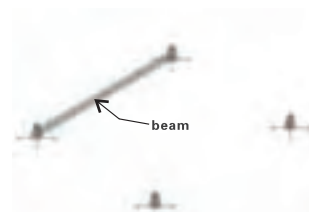
5.Install beam between each 2 pillars
