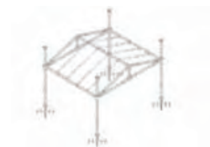
10.Last step: Fix the slant brace on the brace . The opposite way to dismantle it
